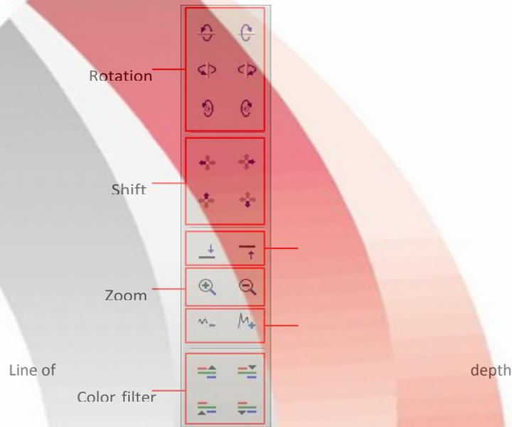
Difference in heightFigure 7: Operating Elements of the Navigation Bar
