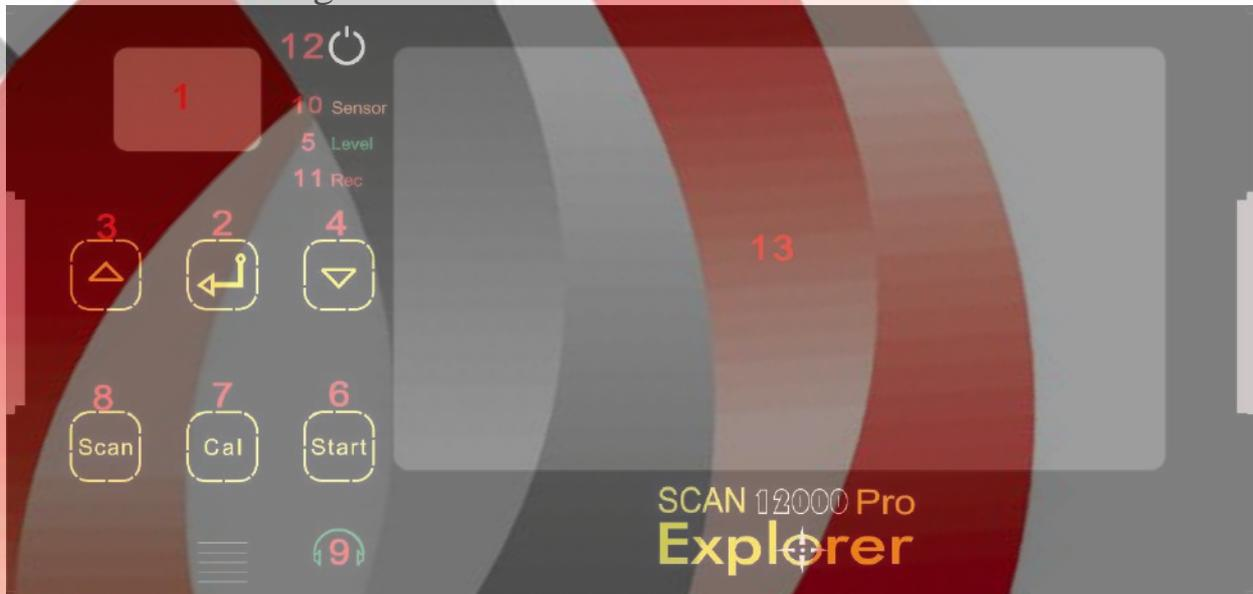
1. Character display for communication and control between the menus and different parts of the machine
