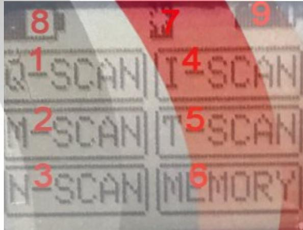
1. Quick scan for automatic scanning audio + magnetometry
